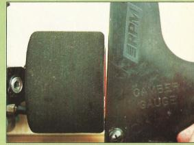
but pressing down on the chassis, as if it were squatting under power or cornering, brings the 'Active' geometry into play, hence the toe-in seen here. Clever!
