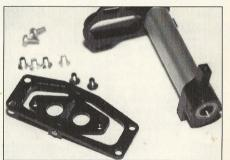
The pivot bracket to which the motor pod mounts. The smaller inner section mounts to the chassis "voke".
