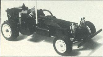
making the chassis assembly rigid. The only work that was necessary to the RC side of the job was to turn the steering gimble on the 'Tamtech' transmitter upside down as the steering was working in reverse. Alternatively turn the servo over or if your transmitter is fitted with servo reverse then flicking the switch is all you need do. Painting and trimming the body was the final task and all is ready for the first run.
