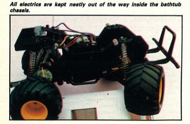
moulded, bathtub type chassis with all the necessary provisions for radio installation, kit speed controller and battery installation. The rear wheel drive is through a
