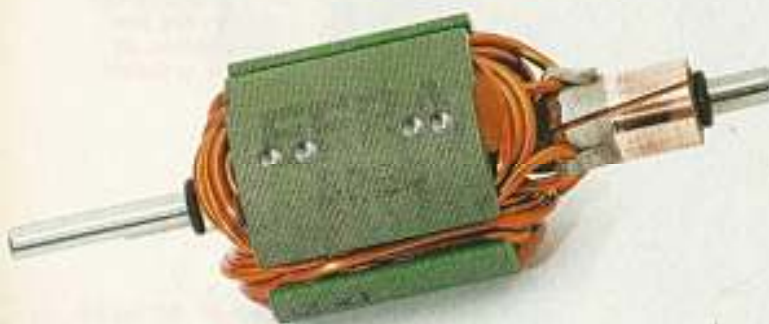
Hand wound, this is how the comm looked after the first runs, and the brushes are only just bedded in
