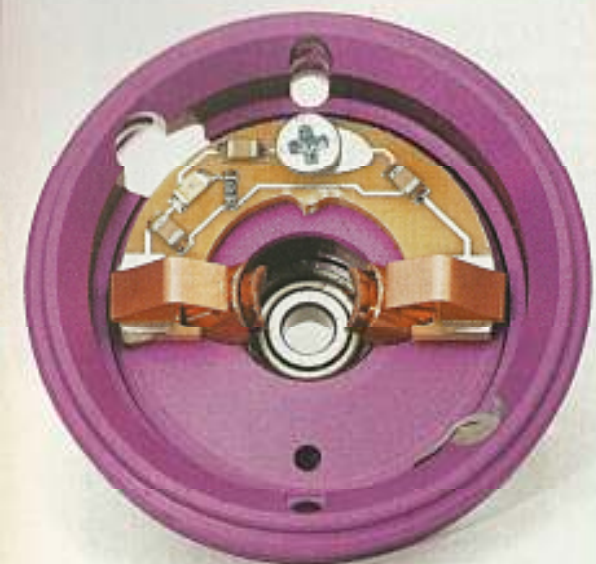
This circuit board is for the capacitors and the various status LED's, also you can just see the insulators for the brush tubes
