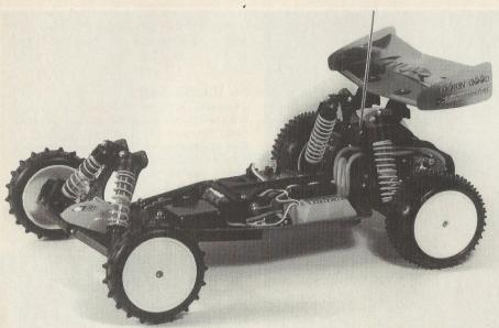
Power to weight. Another means of identifying the 'Works' car is by its proven carbon fibre shock towers, which are fitted both front and rear to reduce weight and marginally lower the centre of gravity. They are identical in shape to the standard glassfibre parts, and like many of
