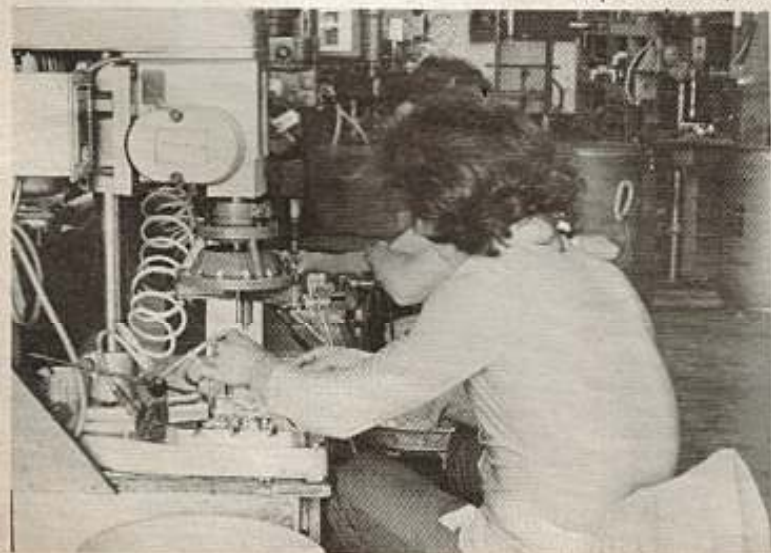
Below left: further automatic machinery is employed, here thread tapping is taking place. Below right: three bays of the factory unit are taken up with storage of bulk parts - how many drivers wouldn't sign away their souls to be let loose in here?
