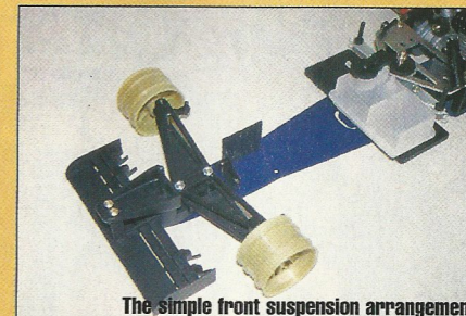
The simple front suspension arrangement
