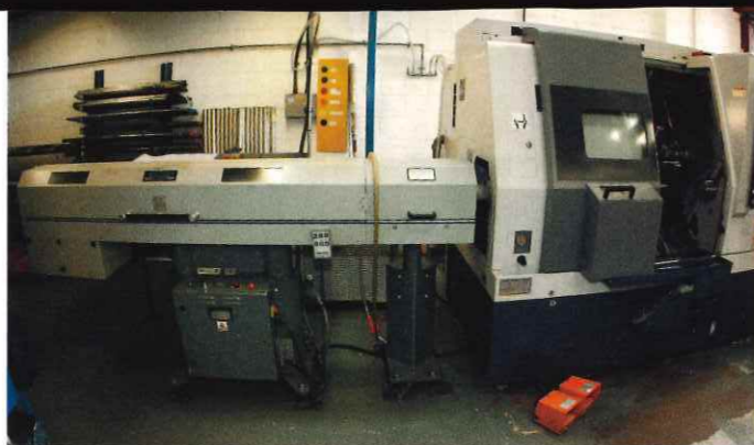
The CNC Mill/Turning Centre with feed stock to the left, requires minimal attention once tooling, set up and programmed
