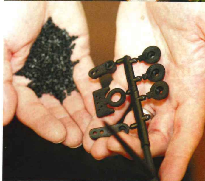
High-pressure moulding machines turn virgin polymer chips into components under extreme pressure
